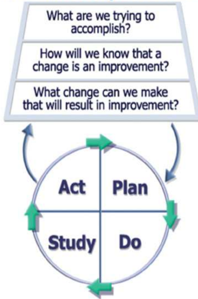
FIGURE 49-2 The Model for Improvement. (From Associates in Process Improvement. Available at http://www.apiweb.org )
