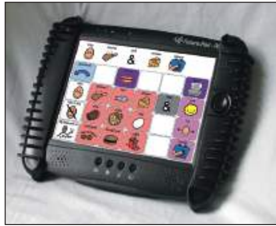
Figure 4.12 An example of a touch screen speaking communication aid to assist children who may have speaking and movement difficulties.
