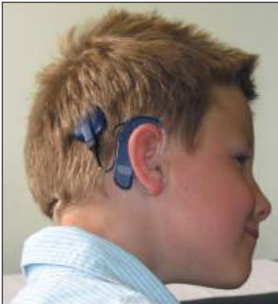
Figure 4.7 Cochlear implant. There is a microphone to detect sound, a speech processor and a transmitter and receiver/stimulator. They convert speech into electric impulses which are conveyed to the auditory nerve, bypassing the ear. It provides a deaf person with a representation of sounds.
