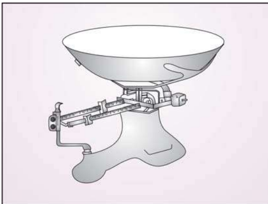
Fig. 3.3: A conventional beam balance scale for weight recording in hospital and clinic practice
