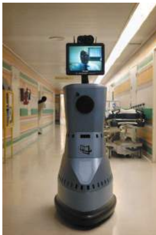
Figure 7.11 Remote presence robot (courtesy of the Department of Biosurgery and Surgical Technology, Imperial College, London).
