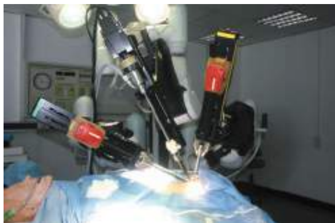
Figure 7.5 Slave unit: da Vinci arms set up in a virtual operating theatre (photo courtesy of Daniel Leff).
