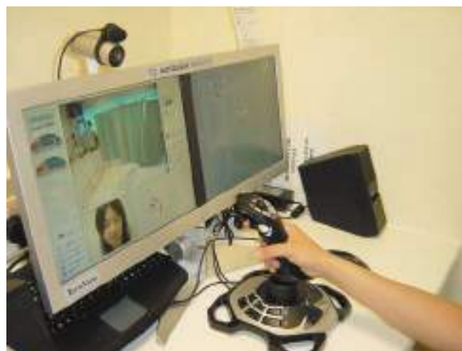
Figure 7.12 Remote presence console (courtesy of the Department of Biosurgery and Surgical Technology, Imperial College, London).
