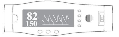
(iii) Pulse oximeter showing good plethysmographic (pulse) wave with low oxygen saturation
