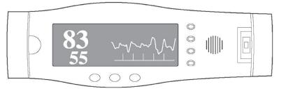
(ii) Pulse oximeter showing a poor Plethysmographic (pulse) wave
