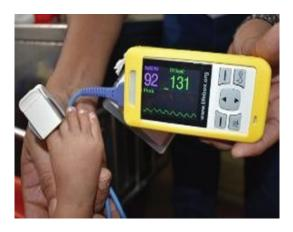
**Step 6:** Allow several seconds for the pulse oximeter to detect the pulse and calculate the oxygen saturation. Once the unit has detected a good pulse, the oxygen saturation and pulse rate will be displayed. Look for the displayed pulse indicator that shows that the machine has detected a pulse. Without a pulse signal, any readings are meaningless.
