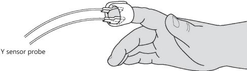
The probes and connecting cables are delicate and are easily damaged if stepped on. Cables break more frequently as the pulse oximeters age. Finger clipon sensors last about 6 months on average and can be used on many children during this time. It is important always to have a spare probe available in case one fails.
