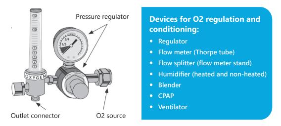
Figure-4: Thorpe Tube flow meter with pressure regulator and outlet connector
